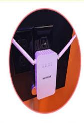
Arrange the Wi-Fi extender's antenna vertically for a better signal.
